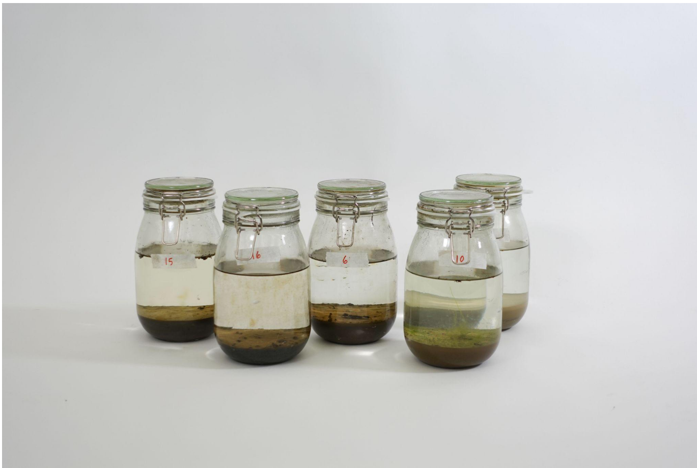
Granulometry test of earth samples from Oslo, Earthly Archive, Earth Matters studio, AHO, 2021.
